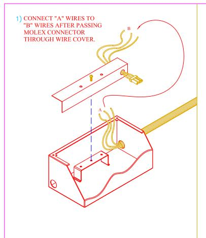
2) CONNECT MOLEX CONNECTOR "A" TO MOLEX CONNECTOR "B" BEFORE MOUNTING BALLAST TRAY.
