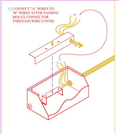
2) CONNECT MOLEX CONNECTOR "A" TO MOLEX CONNECTOR "B" BEFORE MOUNTING BALLAST TRAY.
